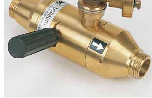
Manufactured from solid brass by AWG in Germany, this inductor can be mounted inline (adjustable) or in a by-pass set up (fixed) between the HP pump outlet and HP hose reel drum inlet to produce an effective foam media.
